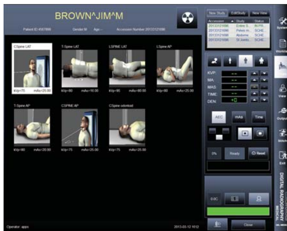
Generator Exposure Control and Positioning Guide
